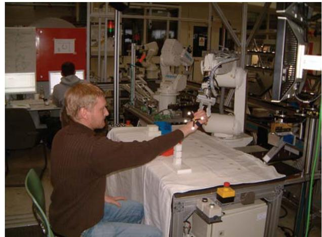
**Figure 8** Picture of the JAHIR robot system while it is assisting a user by an assembling task.
