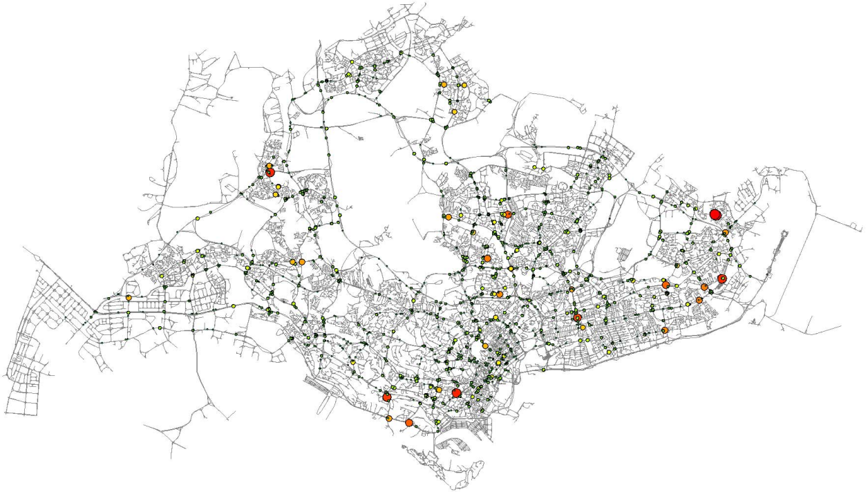
Fig. 5: Spatial distribution of dynamic factor of intersections in Singapore according to simulated agent routes. Big red dots mean high dynamic factor and small green dots mean low dynamic factor. Only intersections with throughput higher than 10000 cars per day are considered.
