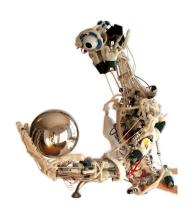
Fig. 1. ECCE, a so called anthropomimetic robot, is the platform for the work presented here. In this type of robot not only the outside of the human body is copied but also the inner structures, like bones, joints, muscles, and tendons.
