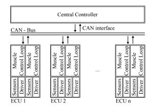
Fig. 4. In a centralized control architecture (Fig. A) like it is used for Kotaro [4] all control is run on a single controller. The control architecture proposed here (Fig. B) distributes fast local control loops into the robot's limbs, while communication with the central controller is accomplished via a CAN bus system.
