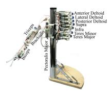
Fig. 6. The anthropomimetic robot arm with 11 AM that was successfully controlled by the proposed control infrastructure.
