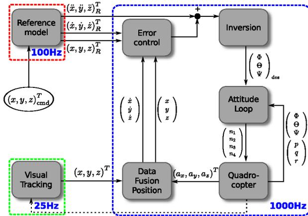
Fig. 2. Structure of the controller including the different processing rates. In the figure,  $x$ ,  $y$  and  $z$  denote the position,  $\Phi$ ,  $\Theta$  and  $\Psi$  denote the bank, pitch and yaw angles.  $p$ ,  $q$  and  $r$  are the respective angular rates in the same order.  $n_1$ ,  $n_2$ ,  $n_3$  and  $n_4$  are the four rotations per minute (RPM) of the rotors, and  $a_x$ ,  $a_y$ , and  $a_z$  are the accelerations obtained from the IMU
