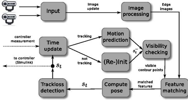
Fig. 3. Flow of the visual tracking system
