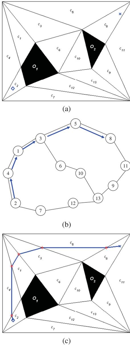
Fig. 2. Main steps for planning a fully-actuated point robot based on cell decompositions. (a) Environment with two obstacles, free space decomposed in triangular cells, start position marked with  $\diamond$ , target position marked with X; (b) Corresponding adjacency graph and a path linking the start and the destination nodes; (c) The robot trajectory corresponding to the graph path (blue); the middle points of line segments shared by adjacent cells are marked with red.
