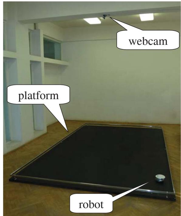
Fig. 1. Experimental test bed that consists of a black platform on which a Khepera III robot moves, and a surveying web camera.
