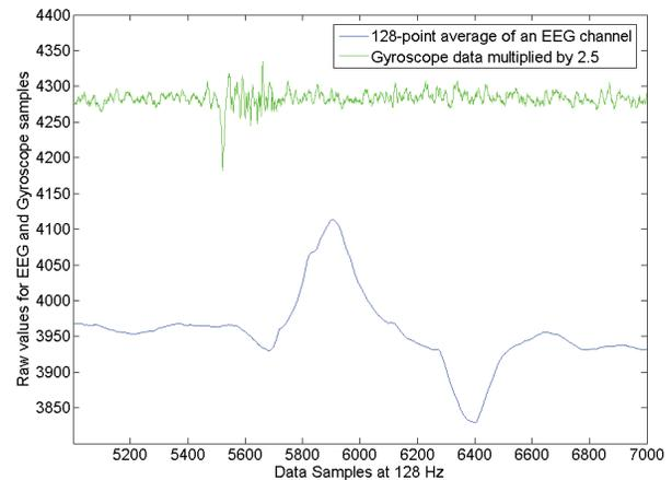
Fig 5. Scaled gyroscopic data and raw EEG data showing how increased gyroscopic Y activity (green) resulted in EEG moving average (blue)
