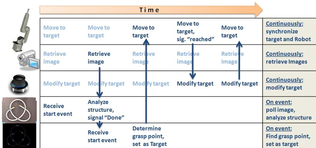
Figure 5. Schema of a subsequence of the introduced demo application workflow<sup>13</sup>
