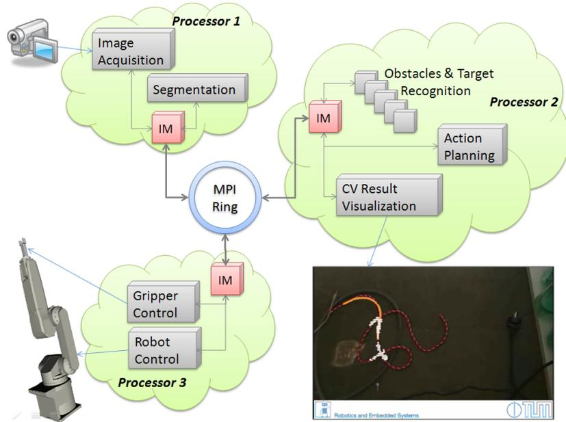
Figure 4. A possible unit setup of the application for limp object recognition and robotic handling. The actual mapping of units to processors and of processors to computers depends on the MPI environment.
