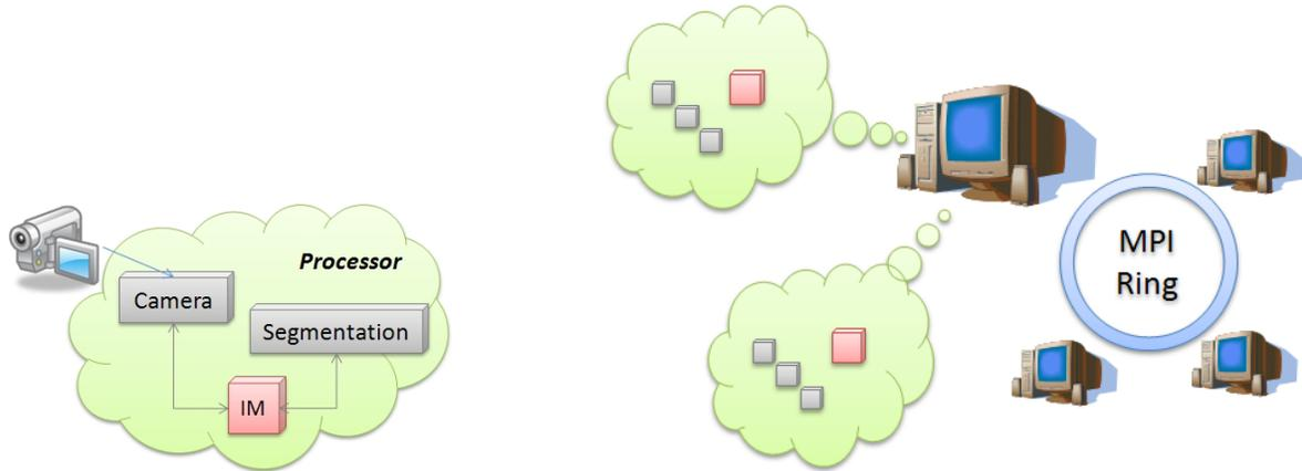
(a) Units are bound to processors at runtime. The user may force binding to a computer by IP-address.
