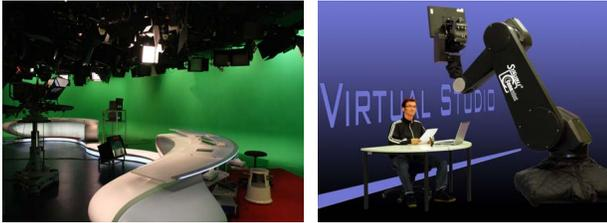
Figure 1: Left: A Virtual Reality TV Studio with manually operated TV Camera (*image courtesy: RTL Television Studio Köln, Germany*) Right: TV Camera operated by a Industrial Robot (6dof) together with a Pan Tilt Unit (2 dof)
