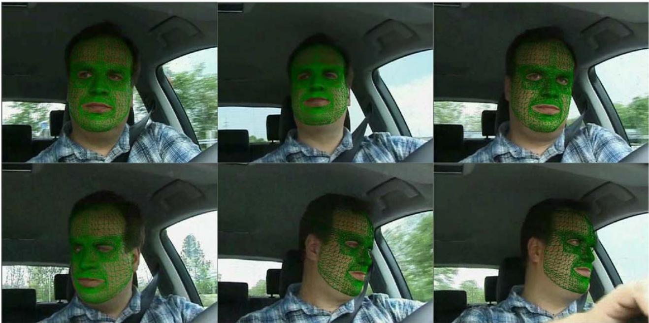
**Fig. 7** Stable 3D head tracking in a car-driving environment
