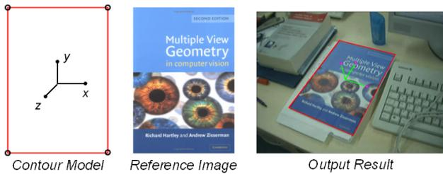
Fig. 8. Contour-based tracking by optimizing local color statistics.
