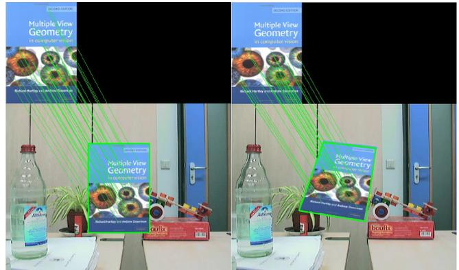
Fig. 7. 3D Pose estimation with invariant keypoints - GPU-based implementation.
