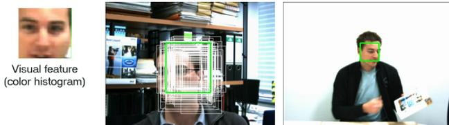
Fig. 5. Color-based particle filter.
