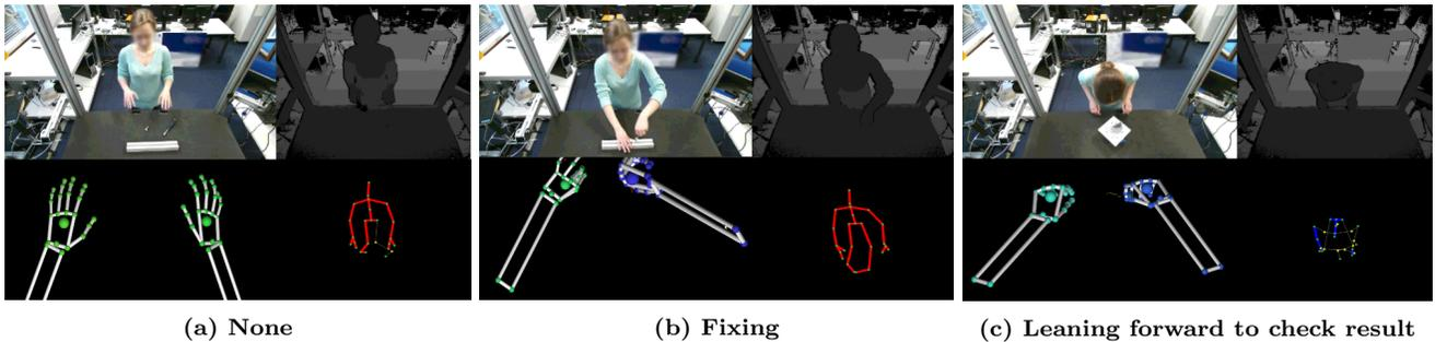
Figure 4: Visualization of multimodal input to the HRI interface. For each of the three exemplary activities, it depicts the RGB and Depth images (top left and top right) from a Kinect v2 sensor, the derived body skeleton (bottom right), and the hand skeletons (bottom left) detected by two Leap Motion sensors.
