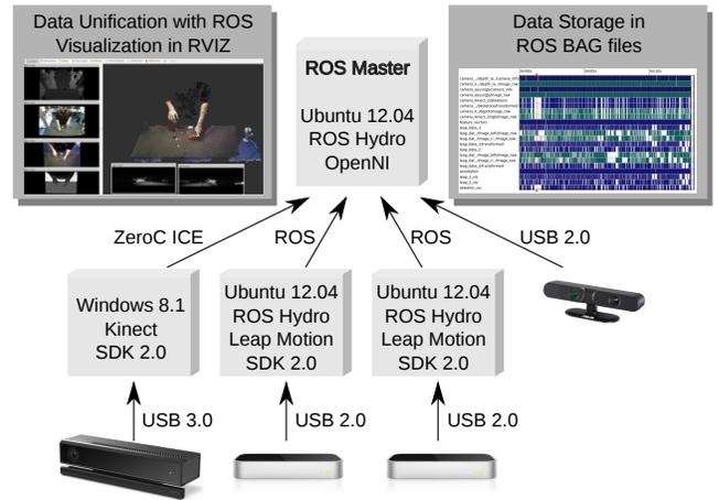
**Figure 3: System overview: communication and control of multiple sensors.**
