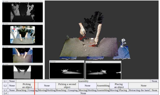
**Figure 1: HRI workcell used for human activity recognition in industrial assembly scenarios. Data from the Asus Xtion Pro sensor is processed into a 3D point cloud and further extended with the finger tip positions obtained by Leap Motion sensors (red arrows). The timeline bar on the bottom shows the suggested multilevel annotation of human activities.**
