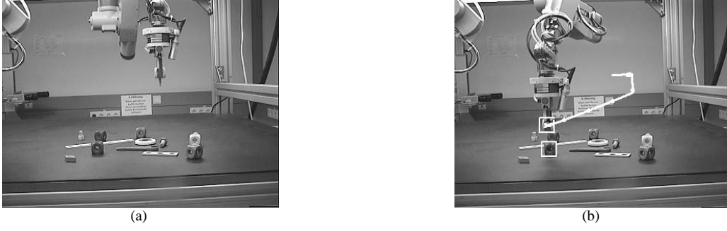
Figure 3. Initial (a) and final position (b) of the manipulator and its projected trajectory as seen from one camera.
