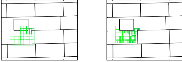
Fig. 2. Before splitting (left) and after (right); green boxes denote the reachable region in the position domain at the current \Delta t ; black rectangles denote obstacles
