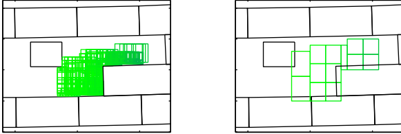
Fig. 3. Before repacking (left) and after (right); green boxes denote the reachable region in the position domain at the current \Delta t ; black rectangles denote obstacles
