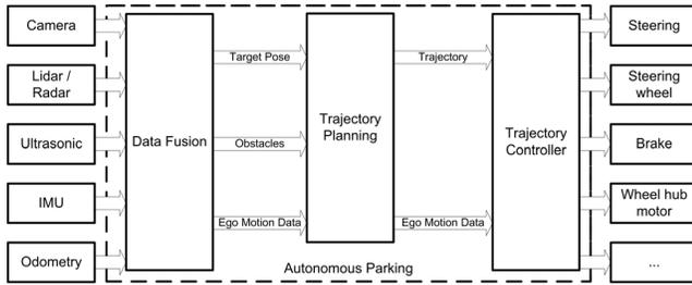
Fig. 5. Software architecture of the autonomous parking function
