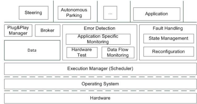
Fig. 2. Layers of the RACE Run-Time Environment (RTE)
