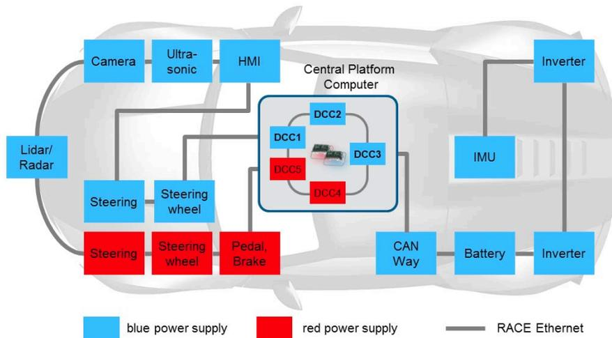
Fig. 3. E/E Architecture with Central Platform Computer
