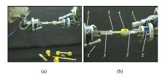
Figure 1: The experimental setup for assembly. 1,1': hand-camera; 2,2': force/torque sensor; 3,3': parallel jaw-gripper; 4: nut; 5: screw.
