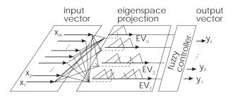
Figure 6: The structure of a fuzzy controller based on eigenspace projection.
