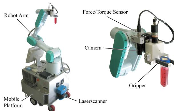
Figure 1: The mobile robot as it was shipped to the customer.
