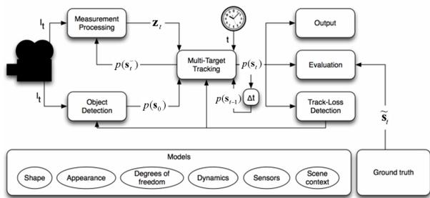
**Figure 3: The flow diagram of our model-based, multi-purpose tracking library: OpenTL.**
