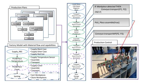
Fig. 2. The workflow for generating action sequences. A valid action sequence is generated from the product and factory descriptions. This is later translated into an executable action sequence.
