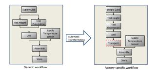
Fig. 1. Transformation of a generic workflow into a factory-specific one.
