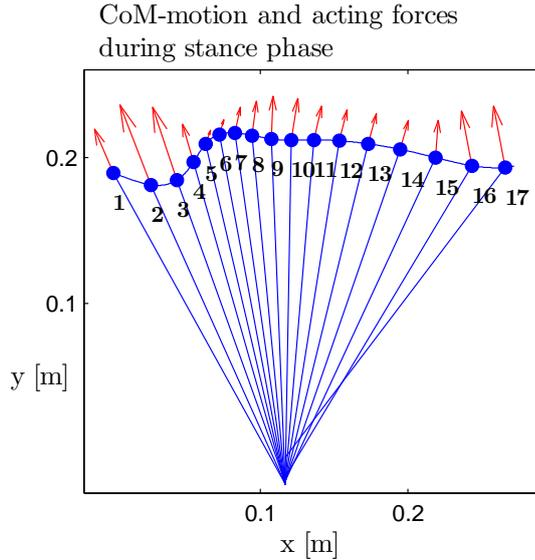
**Figure 2:** Forces acting on the CoM in stance are indicated with arrows pointing in the effective direction of the force at this instant. The length of the arrow corresponds to the relative magnitude of the force. CoM-position and leg orientation are indicated for different instants during stance phase.
