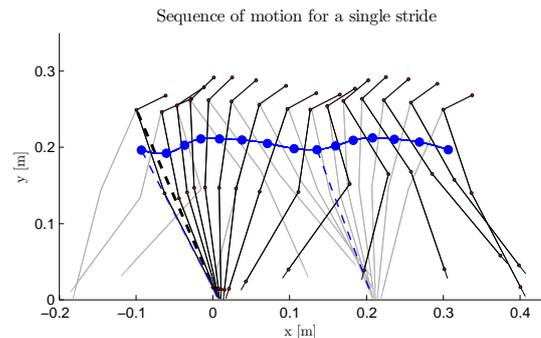
**Figure 1:** Sequence of a single stride, the initial stance leg is indicated in black, the swinging leg in grey. Positions of markers on the initial stance leg are indicated as small circles. The position of the CoM for every frame displayed is indicated by a large circle, the CoM-progression by the connecting line.
