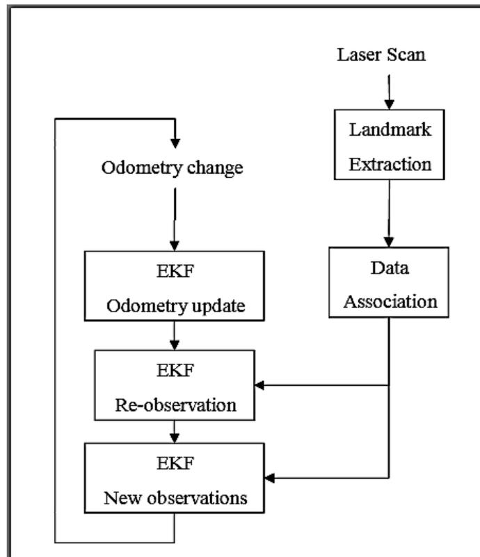
Figure 2.3: *Overview of a typical SLAM process.* The Graph shows the basic process of SLAM done with the EKF algorithm.[12]
