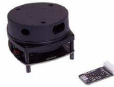
(b) RPLIDAR - 360 degree Laser Scanner
