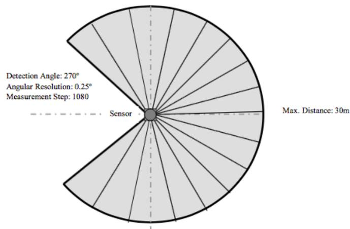
Figure 3.2: *Diagram of scanned area*[17]. It shows how the scanning area of the used LiDAR looks like.
