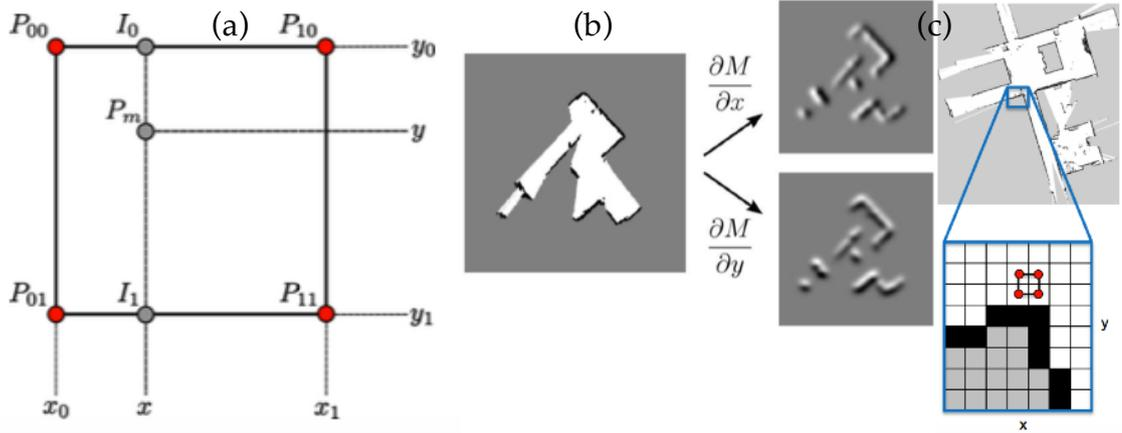
Figure 3.4: *Hector\_SLAM filter method.* „(a) Bilinear filtering of the occupancy grid map. Point  $P_m$  is the point whose value shall be interpolated. (b) Occupancy grid map and spatial derivatives.“[18] (c) A small zoom of the whole grid map.
