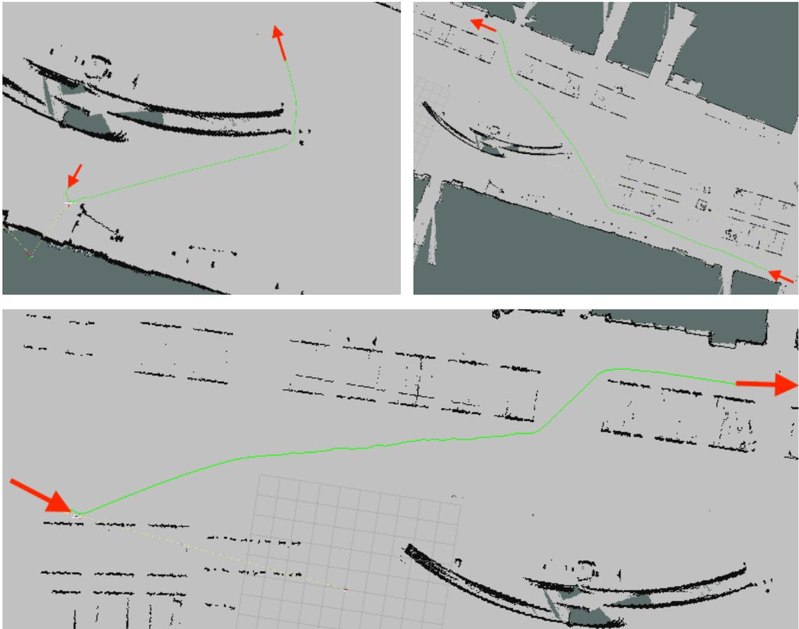
Figure 4.3: *Global routes*. Here are some global routes presented. The green lines are the calculated routes from the estimated starting point (arrows with peak to the lines) to the set goal (arrows with peak away from the lines). The arrow peaks also show the front of the car at the beginning and the end.
