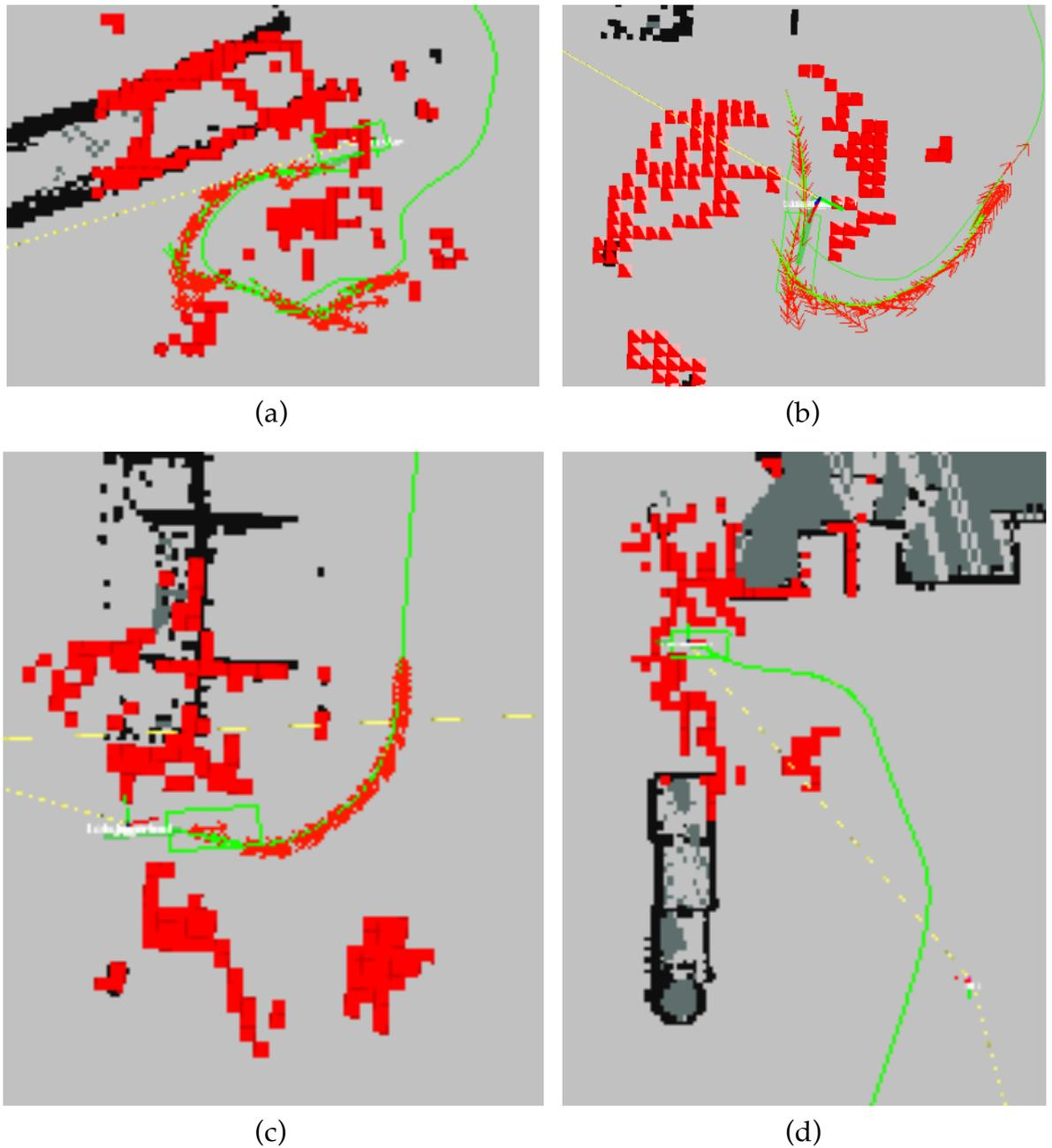
Figure 4.4: *Local routes*. The picture shows four different local routes. Picture (a) and (b) shows the difference between the local and the global route. The green line is the global route and the green line with the red arrows on it is the local route. In (c) the local route is nearly the global route. In (d) they are exactly the same. The red squares are detected obstacles.
