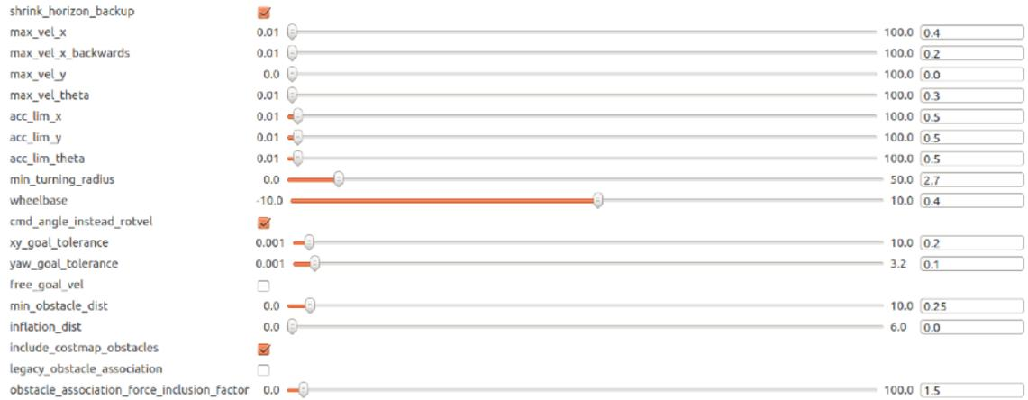
Figure 3.5 Examples of some `teb_local_planner` arguments. This picture shows a few of the required parameters for the `teb_local_planner`
