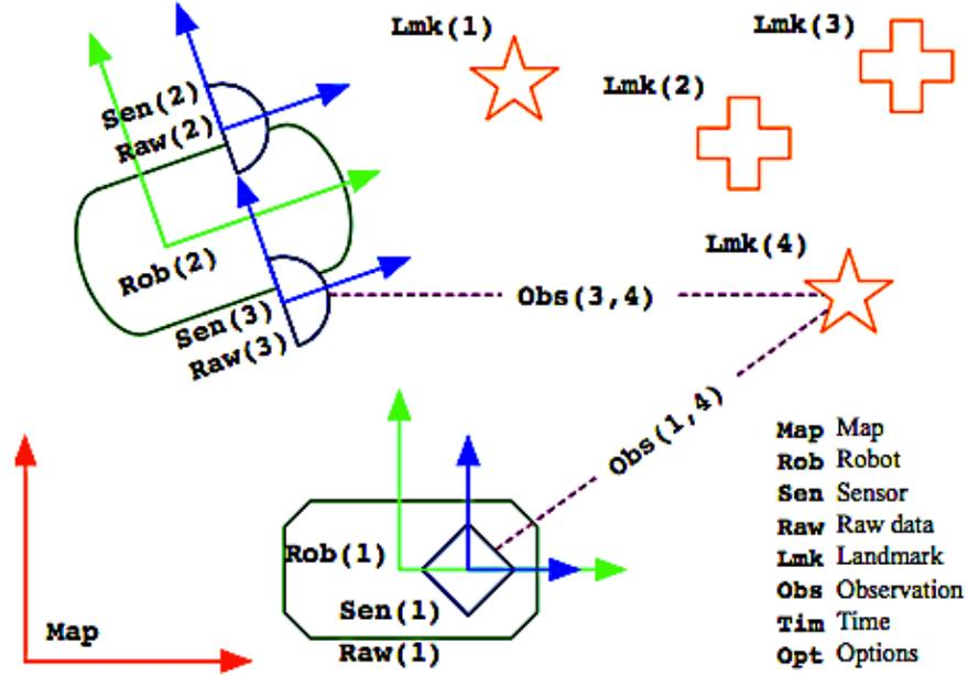
Figure 2.4: *Typical SLAM entities.*[16] The picture gives a good example how the sensor information is filled with an angle and a distance to an obstacle. Robot(1) detects landmark(4) at the initial pose, then it moves on to robot position (3) and it still detects the landmark (4) but with another distance and angle.
