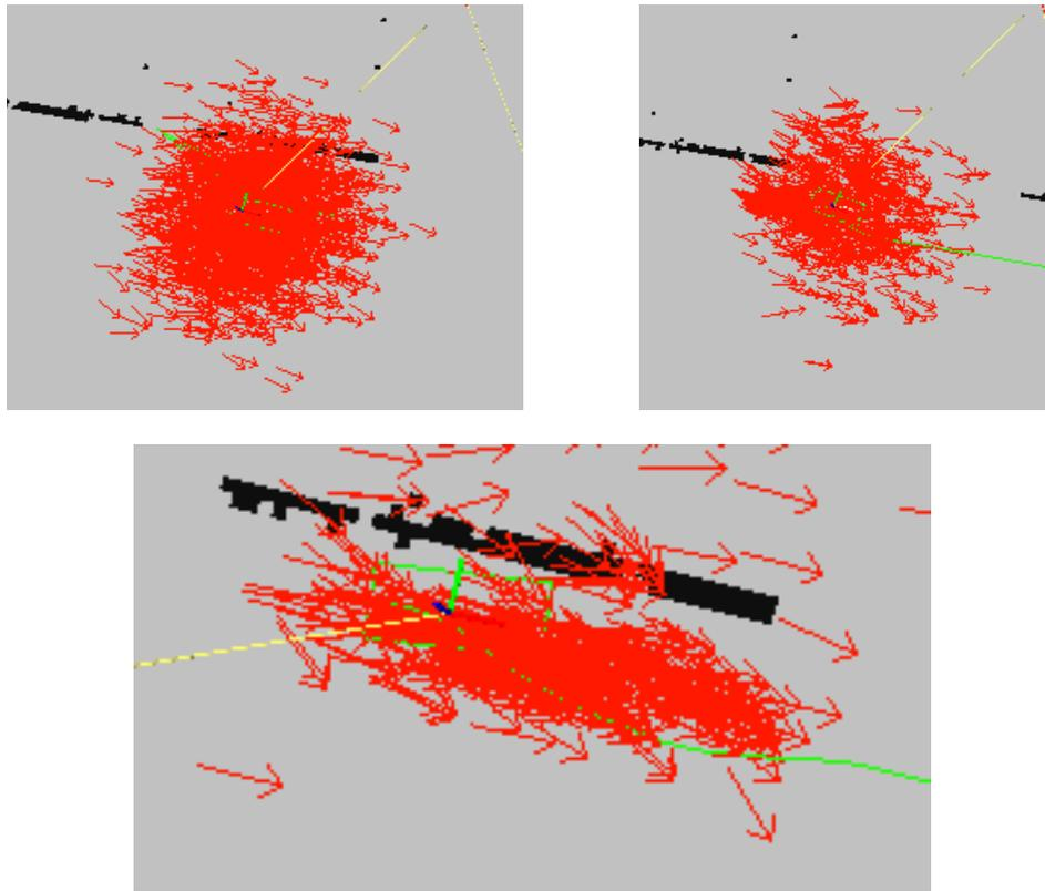
Figure 4.5: *Localization array*. The picture shows the step by step localization during the car's driving. At the beginning the estimation cloud is very big, but as soon as the car starts driving the estimation gets more precise.
