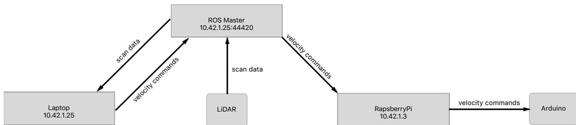
Figure 3.3: *Basic relation model of the hardware.* This graph shows the relation between the different hardware used for the car.
