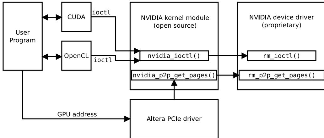
Figure 5.3.: Communication between CUDA/OpenCL and the NVIDIA driver
