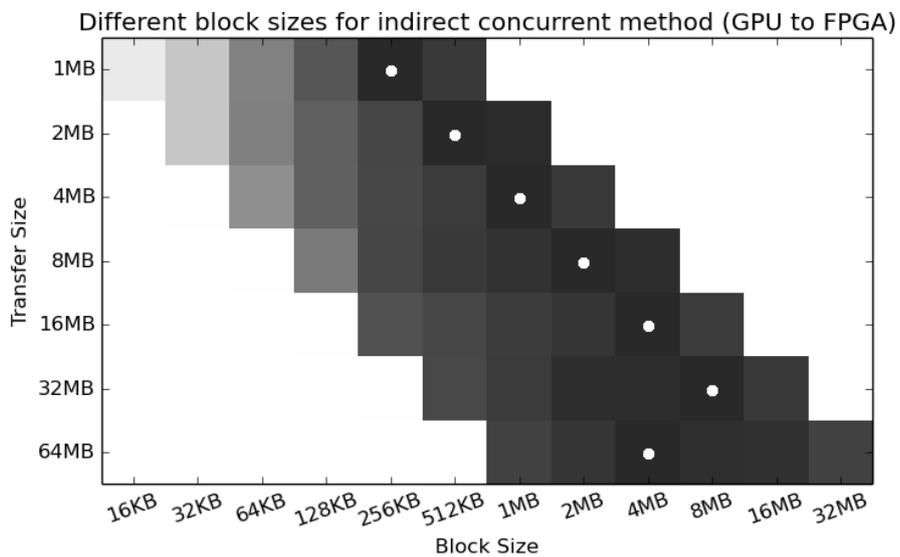
Figure 7.2.: Influence of the block size parameter on the performance for the concurrent indirect transfer method. Higher bandwidth is darker. The white dots mark the maximum bandwidth for each transfer.
