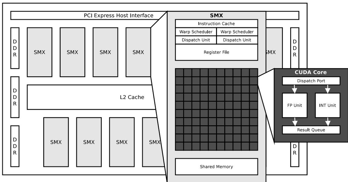
Figure 2.1.: Simplified schematic diagram of the NVIDIA GK110 class GPU architecture. (Image based on [13])
