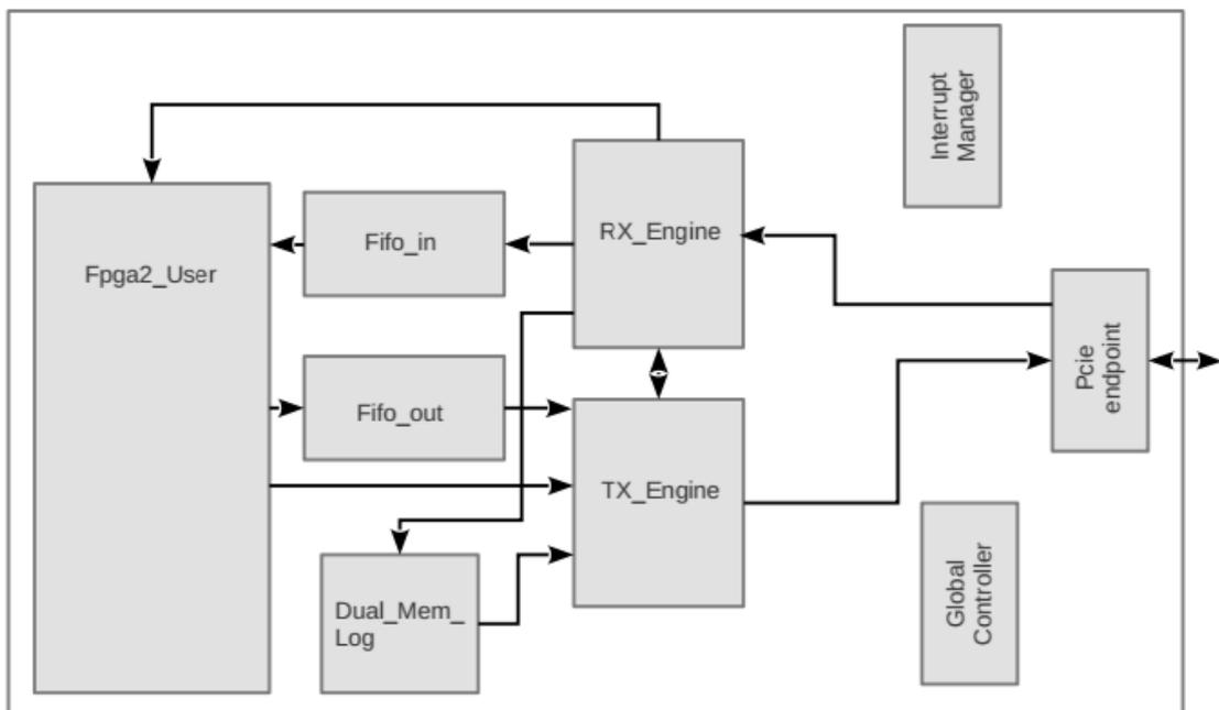
Figure 3.2.: FPGA<sup>2</sup> IP stack design (Image from [33])
