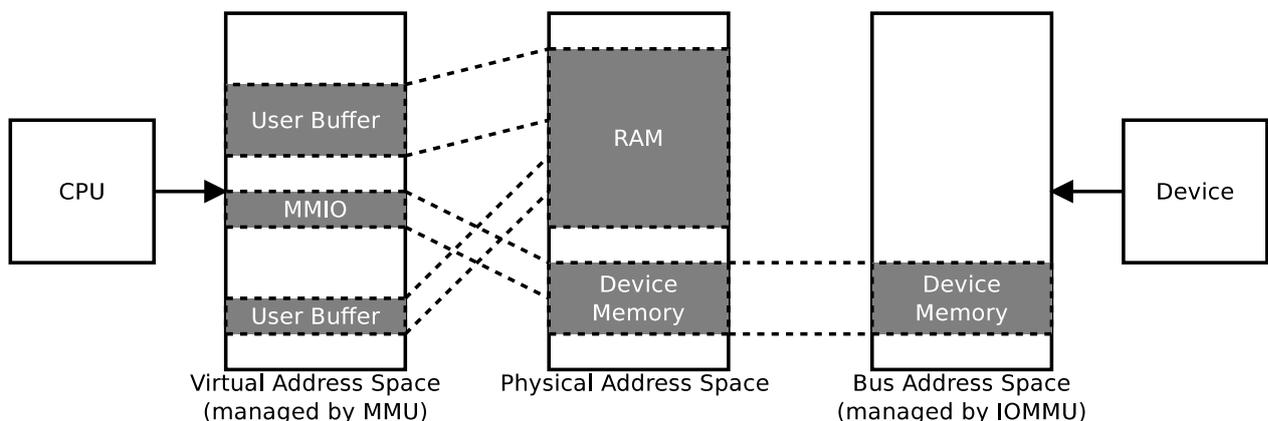
Figure 2.7.: Relationship between the different address spaces with example mappings. In this case the IOMMU performs a 1:1 mapping. (Image based on [32, 29])
