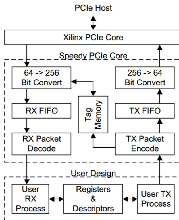
Figure 3.1.: Speedy PCIe IP core design (Image from [8])
