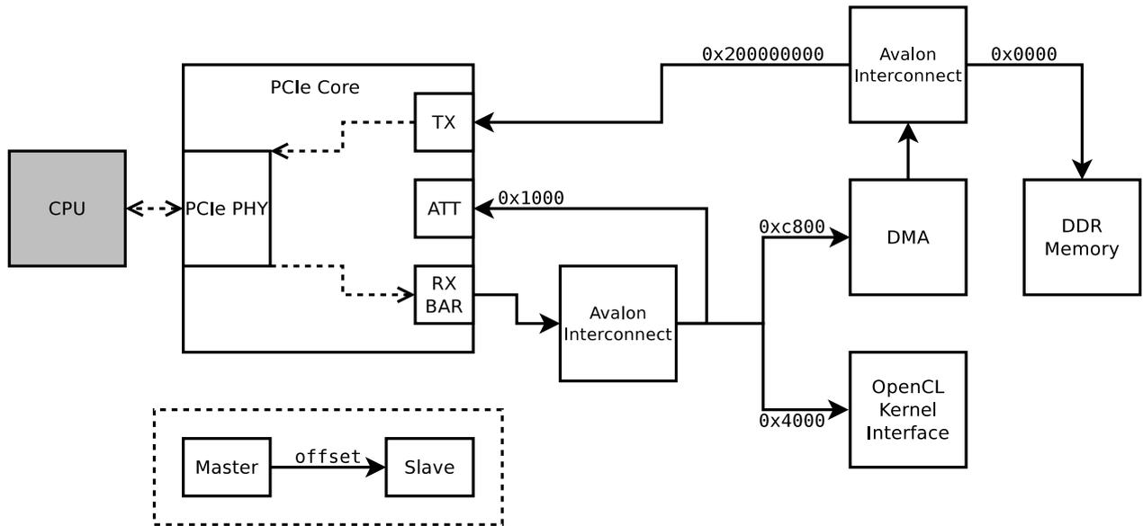
Figure 5.1.: Simplified configuration of the Altera OpenCL IP stack on the FPGA. Note that the solid arrows represent master/slave relationships and not necessarily the data flow direction.
