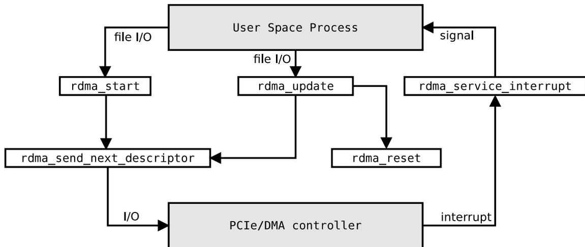
Figure 5.2.: The main functions of the new RDMA component
