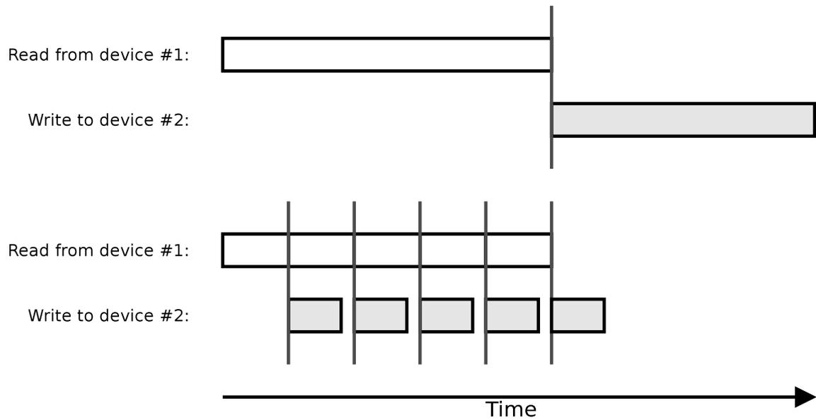
Figure 6.1.: Comparison of sequential (top) and concurrent (bottom) indirect transfer strategies. The two large transfers are splitted into 10 smaller transfers, 8 of them can be performed simultaneously. The gray vertical lines represent synchronization barriers.
