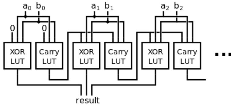
Figure 2.3.: A ripple-carry adder implemented using only 3-input LUTs
