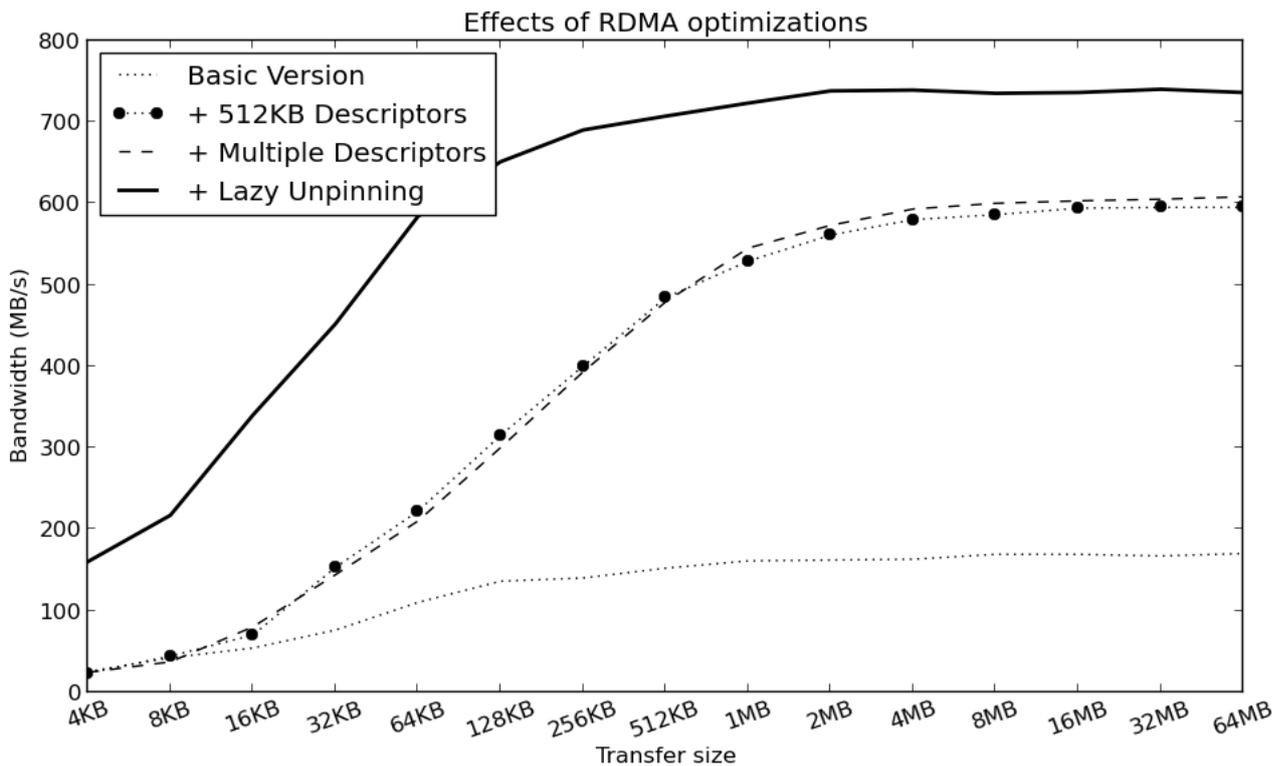
Figure 7.1.: Comparison of the optimizations described in section 5.3.2. Each optimization is added to the previous version (i.e. the Lazy Unpinning benchmark also includes the Multiple Descriptors and 512KB Descriptors optimizations). The Lazy Unpinning benchmark does not include the first transfer, which performs the actual memory pinning.
