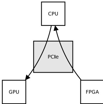
Figure 1.1.: *Indirect* GPU-FPGA transfer
