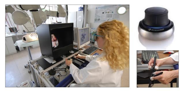
**Description**: We have developed and evaluated a robotic system for minimally invasive surgery. The system can be controlled by haptic input devices that fed back forces to the user.
