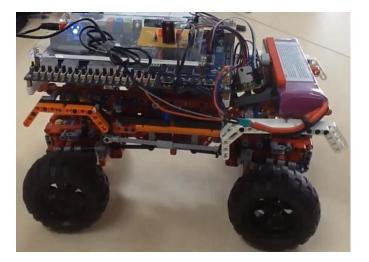
**New Configuration** It has Four DC and Four Servo Lego Motors
