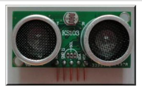
Operate Voltage: 3.0-5.5V; Operate Current: 1.6-2.7 mA typical , 10.6mA max. Standby Current: 500uA, max (I2C mode)
