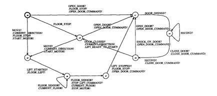
Fig. 5. The lift automaton shown by Autograph.
