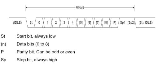
IDLE No transfers on the communication line (RxD or TxD). An IDLE line must be high.
