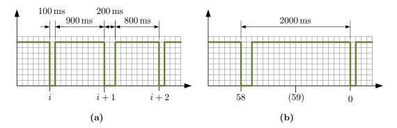
Figure 1: DFC77 Signal Plot: (a) Second mark: binary zero on the left side (100 ms low followed by 900 ms high) and binary one in the middle (200 ms low followed by 800 ms high); (b) Minute mark: there is no low signal in the 59th second.
