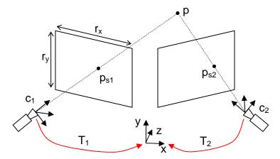
The ball  $\mathbf{p}=(x,y,z)$  describes a parabolic trajectory during the flight, and its motion model can be described by a constant gravity acceleration towards the bottom (-g) + a small random component w (e.g. air resistance in different points of the trajectory). This motion (described in Lecture 4 - Slide 10) gives a probabilistic state model:  $P(\mathbf{s}_t|\mathbf{s}_{t-1}) = \text{Gauss} (A \mathbf{s}_{t-1}+\text{C}, B\Lambda_w B^T)$ .
