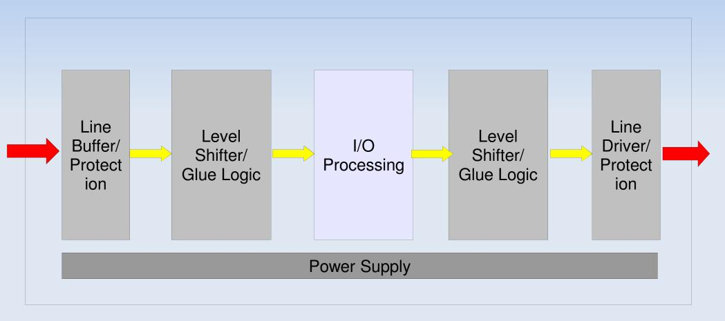
Protective circuits can contain both transient, over/undervoltage protection and galvanic isolation.
