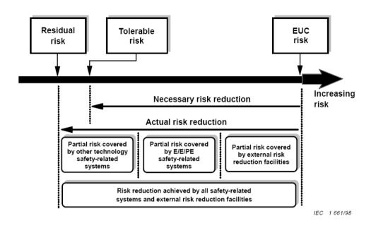
EUC (from IEC61508): System under control E/E/PE (from IEC61508): Electrical/electronic/programmable electronic system
