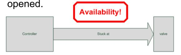
Delivery valve does not open (stuck at failure mode). The process can not be excuted correctly and the product is degraded. The customer is annoyed and a downtime is necessary to clean up the mess.
