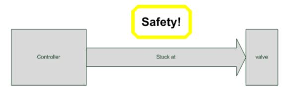
Pressure relief valve does not open (stuck at failure mode). The reactor explodes and people die.
