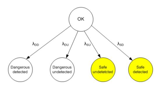
Failure (this is the same failure rate as in the reliability lecture) can happen in a safe or dangerous way.
